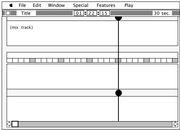
The Mix Control Track controls the playback levels of the two Audio Tracks. Those levels are allowed to change over time. This can be used to reduce the volume on the music when the narrator is speaking.
