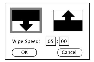
The wipe direction is chosen by clicking on one of the direction icons. The selected icon is highlighted by a colored border around it's outside edge. The white area of the wipe icon represents the image to the left in the Program Sequence. The black area represents the image to the right.
