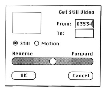
A frame number between 1 and 54000 can be typed in the text entry boxes. If the **To:** number is left blank, then a single icon is produced. If **To:** is fill-in, then a number of icons are produced, one for each frame in the range. The **To:** number must not be less than the **From:** number. An icon looks like a miniature of the still image it represents.
