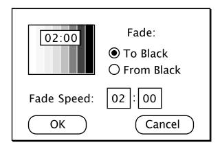
0 to 99 seconds can be entered in the left box. 0 to 29 frames can be entered in the right box. The time entered is displayed in a box in the icon. The **Fade to black** icon has an eight step gray scale going from white on the left to black on the right. The Fade from black icon has the gray scale going from black to white.
